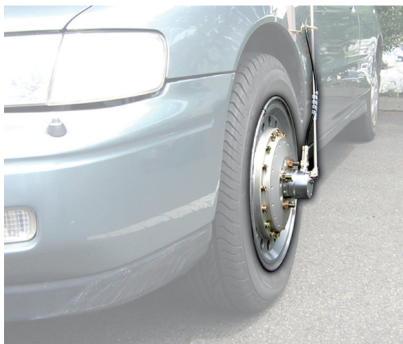
Wheel force transducer with built-in slip-ring and encoder
