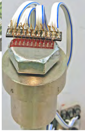
10-element chain type strain gauges on bolt head
